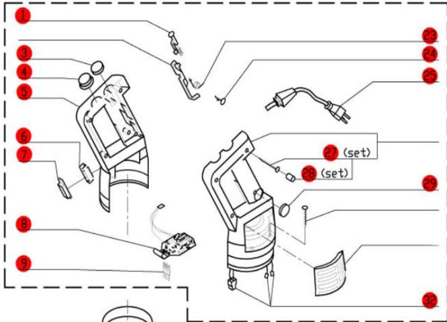
All parts within dashed lines are shipped with replacement screw caps.
